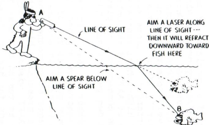
TONTO SHOULD AIM DIRECTLY AT THE FISH HE SEES. IF HE WERE INSTEAD THROWING A SPEAR, HE'D HAVE TO COMPENSATE FOR THE REFRACTION OF LIGHT AND AIM BELOW THE OBSERVED FISH. BUT NOT IF THE "SPEAR" IS A LIGHT BEAM! A LIGHT PATH IS REVERSIBLE, AND WILL GO FROM A TO B ALONG THE SAME PATH IT TAKES FROM B TO A.
